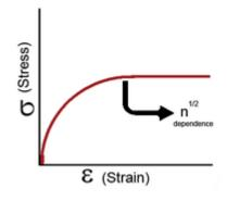
Elastoplastic material is a model for easily plastically deformed materials that simplifies the calculations significantly
