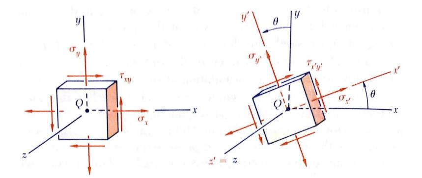
If the material is rotated through an angle  $\theta$  about the z axis, the stress components change to  $\sigma_x', \sigma_y', \tau_{xy'}'$  which can be expressed in terms of  $\sigma_x, \sigma_y, \tau_{xy}$  and  $\theta$
