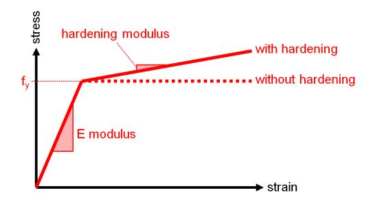
Calculation of the plastic deformations similarly to elastic deformations using Hooke's law is only possible by using a dynamic modulus which is a definite function of applied strain
