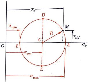
The point A where the circle intersects the horizontal axis is the maximum value of the normal stress  $\sigma_{\chi}'$  and the other intersection point B is the minimum value. Both points correspond to a zero value of shear stress  $\tau_{\chi'\gamma'}$ . These are the principle stresses.
