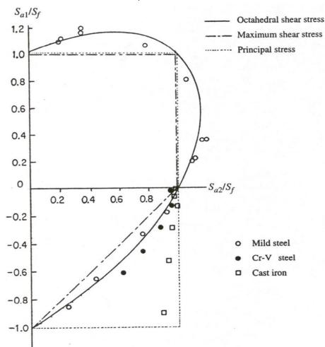
The data for the mild steel and Cr-V steel which behave in a ductile manner agree well with the octahedral shear stress (von Mises) criterion
