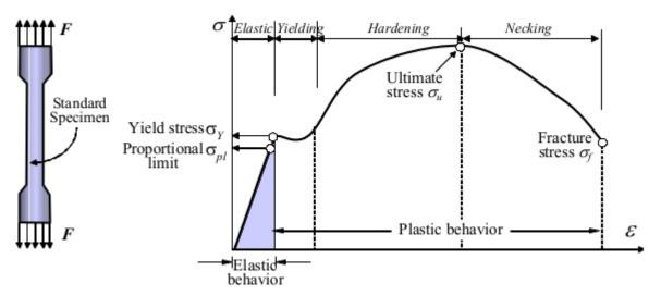
Because dislocation motion is hindered, plastic deformation cannot occur at normal stresses. The yield stress increases as a result.
