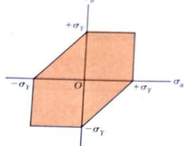
Maximum distortion energy criterion is based on the determination of the distortion energy in a given material, which is the energy consumed by a change in the shape of the material.
